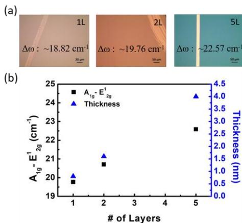
Figure 1. (a) Representative OM images of MoS<sub>2</sub> and (b) their thickness plot measured by AFM and Raman spectroscopy.
